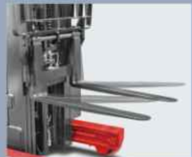
Forks can tilt forward/backward for easy loading
