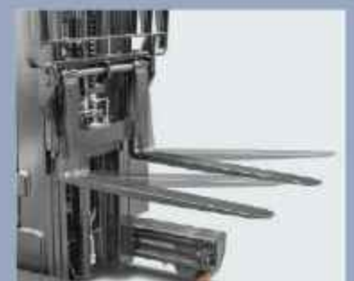
Forks can tilt forward/backward for easy loading
