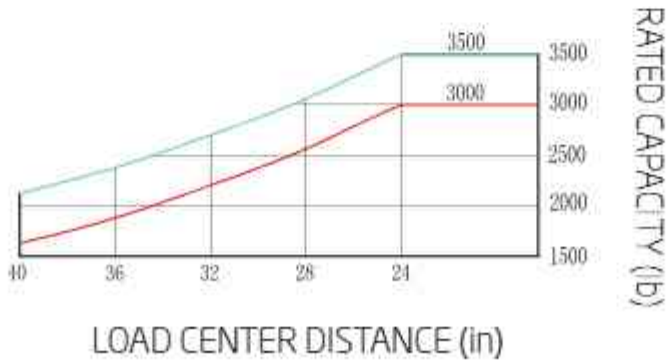
RATED CAPACITY AND LOAD DIAGRAM
