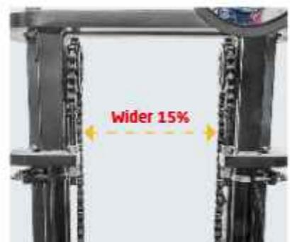
Adopt the new-type of box iron. Increase the inside width of inner mast and the spacing between lifting cylinders. The lowering of instruments in the cabin will greatly increase the forward visibility. The rear visibility will also be greatly improved through the optimization design of counterweight.
