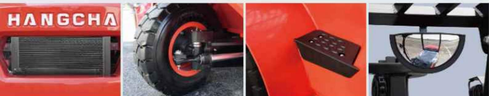
The radiator adopts aluminous plate-fin radiator with better performance and higher structural strength. Impendent oil radiator, optimized oil and water heat dissipation channel and double ventilation holes on counterweight can greatly improve cooling efficiency and reliability of overloaded operation and ensure reliable operation of the engine.
