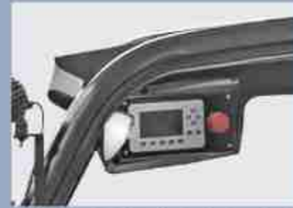
The dashboard in the driver's cab is placed overhead and can be seen when the driver lifts his/her head, and the function buttons can be pressed easily.
