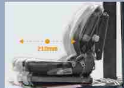
The seat can be adjusted back and forth by 210mm. The operator can choose the best sitting position.
